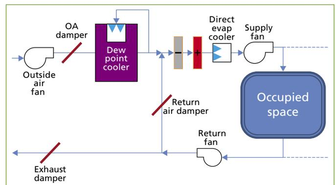
Figure 4. HVAC Configuration SC 2b: VAV system with dew-point cooler and direct evaporative cooling.
