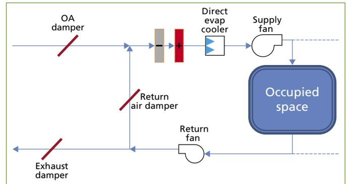
Figure 2. HVAC Configuration SC 1: a conventional VAV system, used as the baseline scenario.
