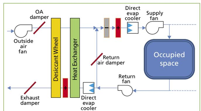
Figure 5. HVAC Configuration SC 3: VAV system with direct/indirect evaporative cooling and a desiccant wheel.
