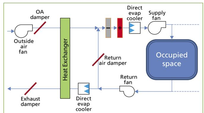
Figure 3. HVAC Configuration SC 2a: VAV system with direct and indirect evaporative cooling.
