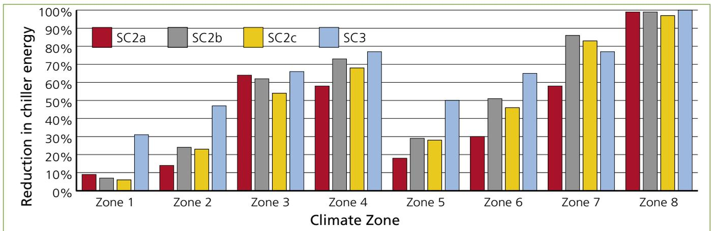
Figure 10. Simulated reduction in chiller energy relative to SC 1.
